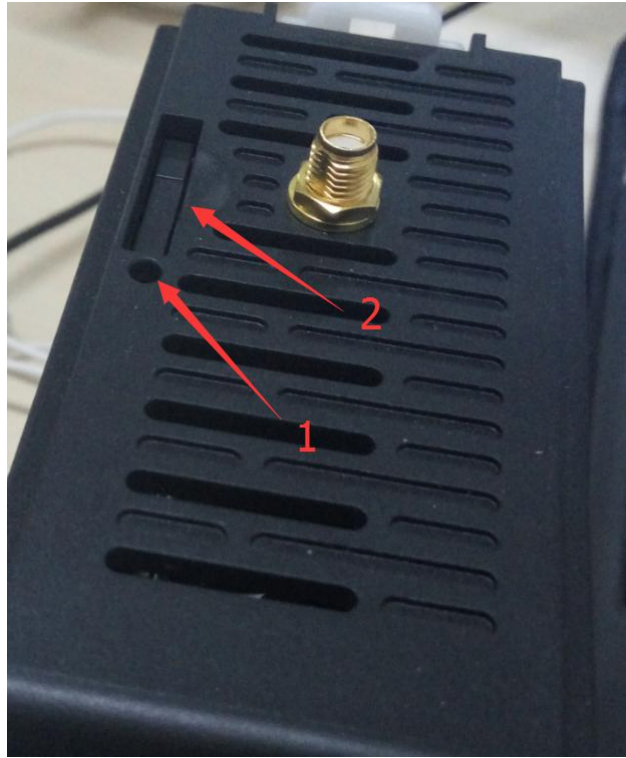
1 keyhole, 2 SIM card slot
